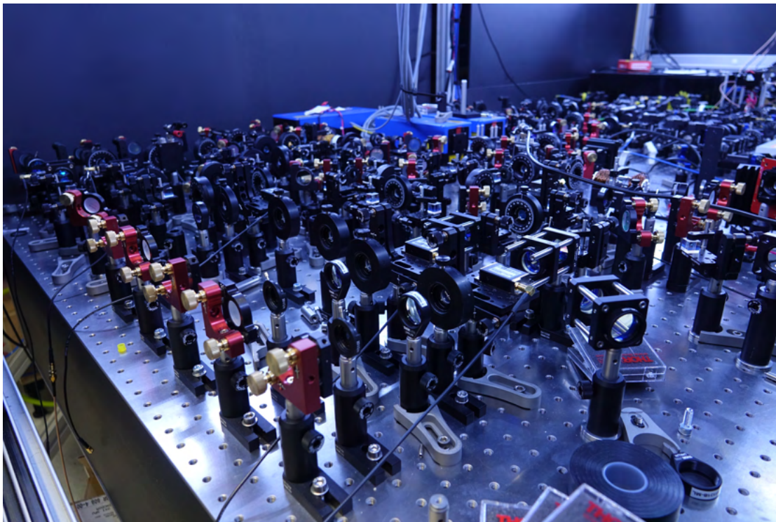
Figure 3.5 – A photo of the K optical setup. At the beginning of the year only a handful of waveplates and AOMs were on the optical table in addition to the lasers and TA (blue boxes).
