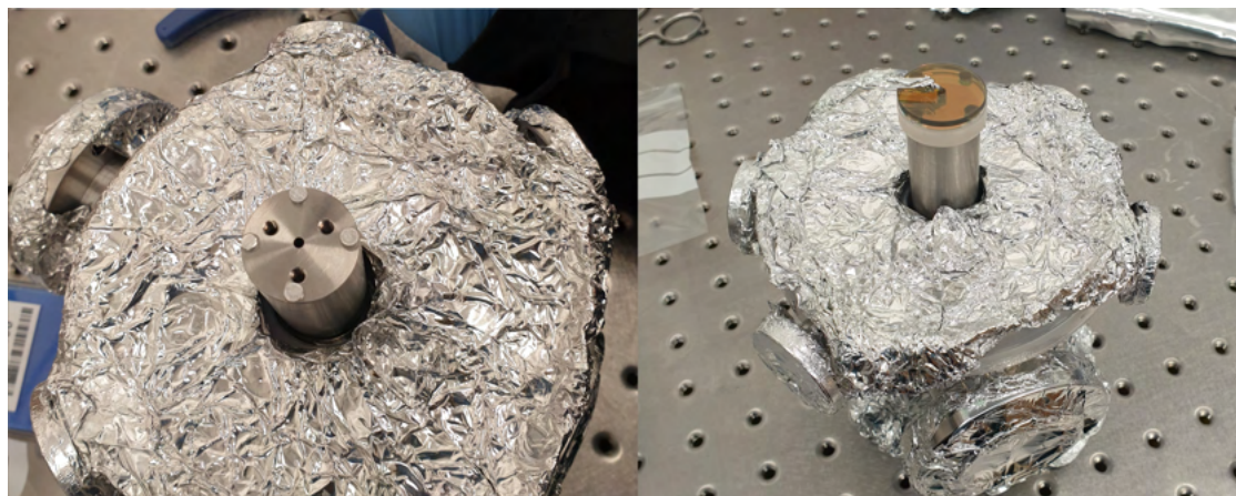
Figure 3.11 – Gluing process - attachment. (Left) First four aluminium spacers were placed at the end of the differential pumping tube. Notice the 2 mm hole in the center that leads to the UHV section. (Right) All components are assembled and aligned using an allen key. In hindsight, the size of the spacers could have been chosen a bit smaller. Also notice the plastic cover sticking out of the aluminum foil in the middle section. This oversight was soon to be regretted.
