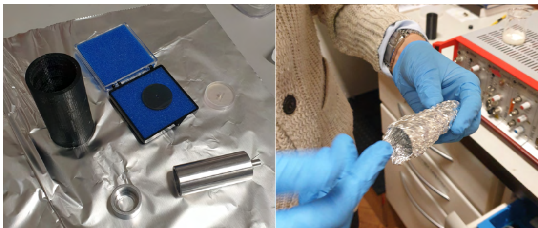
Figure 3.10 – Gluing process - desiccation. (Left) Custom modelled 3D printed cup (black) was planned to hold the glue during desiccation but proved to be incompatible with vacuum. The picture also shows the drilled and coated mirror and polarizer as well as two custom made aluminium pieces that serve as a holder for the K ampoule in the bellow. (Right) Final version of the glue holder made from a hand-shaped piece of aluminium foil.
